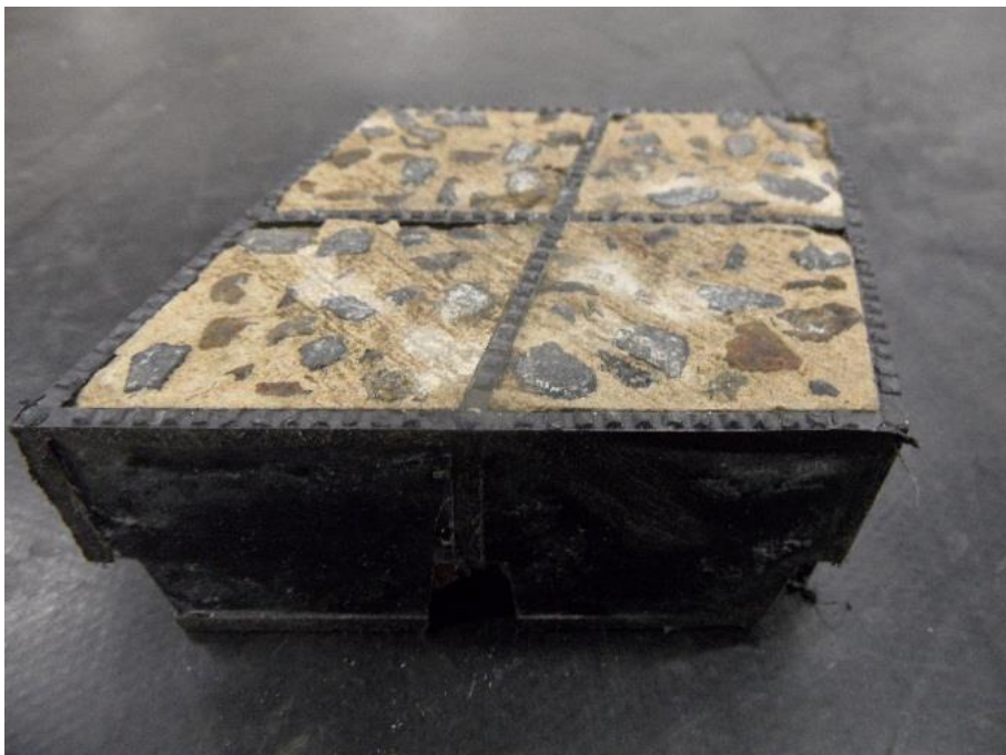
Figure 4: Testing configuration c - The compression of an alternate configuration was cut from the sheet to encompass four cells that are constrained about the perimeter.
