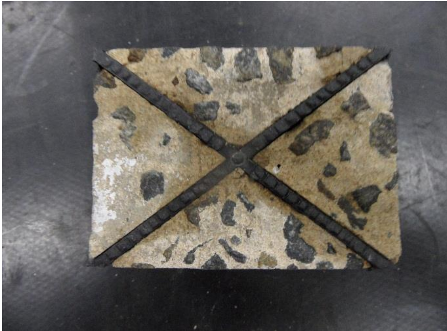
Figure 3: Testing configuration B - The compression of an alternate configuration was cut from the sheet to encompass four cells not constrained about the perimeter.
