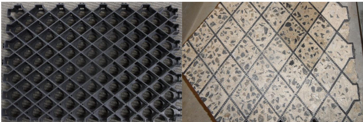
Figure 1: Sheetting before infill is applied. Sheetting after concrete infill is applied (as supplied to ALS)
